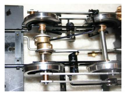
Insert a set screw in the eccentric and screw it in with a 1.5 mm hex wrench until it is nearly tight.
