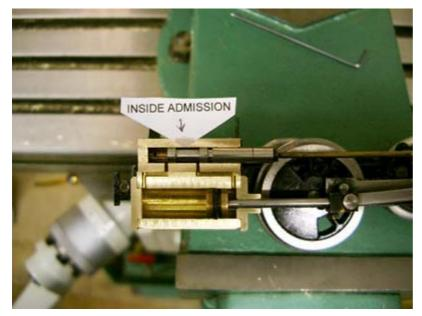
After rotating the eccentrics 180 degrees the engine is now operating with inside admission in forward. Instead of steam pressure pushing the valve out of the block as it does with outside admission, there is only whatever pressure is left in the exhaust applying pressure to the valve linkage and eccentrics. You can also see how the steam moves from the wide groove through the passages to the rear of the piston. The steam then pushes the piston forward and rotates the driver through the rod.
