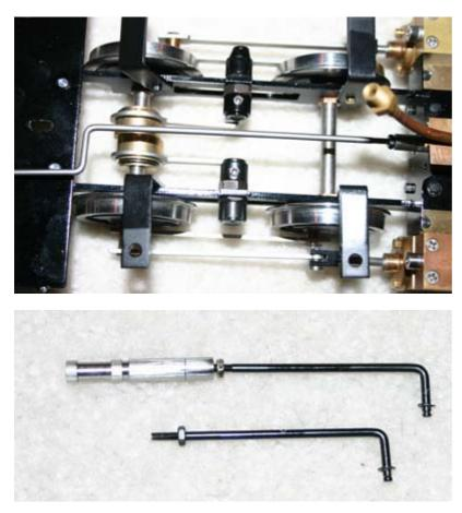
Using a 1.5 mm hex key, screw a stainless set screw into the hole in the inside rocker arm. The photo shows set screws protruding from both rocker Arms.
